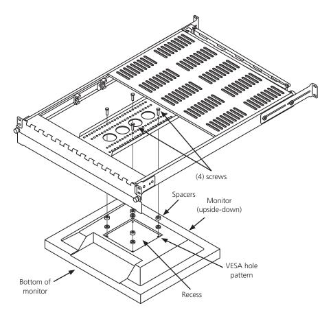
Figure 6. Attaching the monitor.
